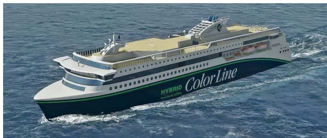
Color Line has signed an agreement with the Norwegian builder Ulstein Verft for the construction of a new 'plug-in' ferry, pictured above, which claimed to be the largest of its kind in the world. Capable of carrying up to 2,000 passengers and 500 cars, the hybrid ferry is designed to operate in environmentally sensitive areas using batteries that are recharged from shore facilities and by the generators onboard. Due to come into service in summer 2019, the ship is destined to operate on the service between Sandefjord and Stromstad.
